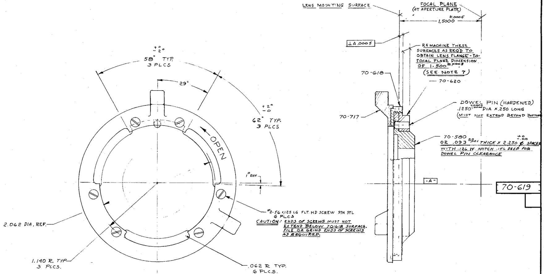
7. ASSEMBLE TO 70-603 GEAR BOX WITH COMPLETED APERTURE PLATE ATTACHED. MEASURE FLANGE DEPTH AND REMACHINE SURFACES INDICATED ON LENS MOUNT RING 70-620 TO GIVE FLANGE DEPTH DIMENSION OF  $1.500 \pm .0005$
