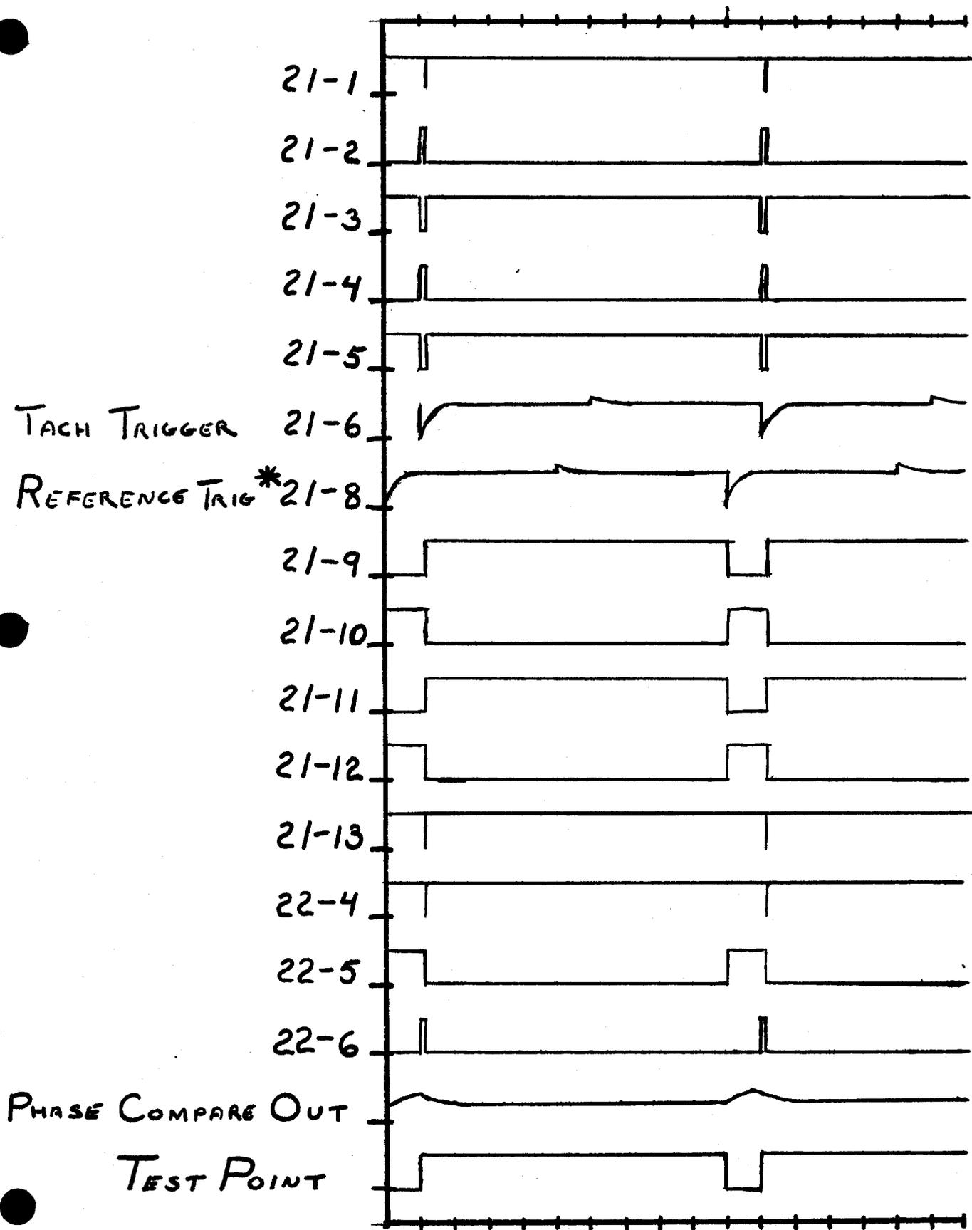
\* SYNC THE OSCILLOSCOPE TO THIS TRIGGER.
