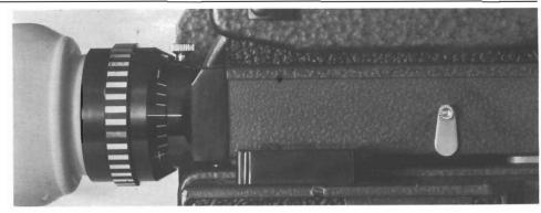
The reflex prism deflects, into the viewfinder, about 25% of the light passing through the lens. The "Exposure times" table on page 12 makes allowances for this in the column "Photometric exposure times".
